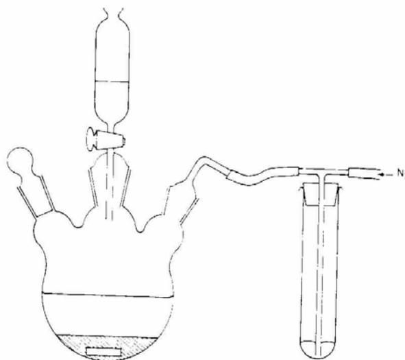
**Figure 1. Apparatus for the preparation of ferrocene**
